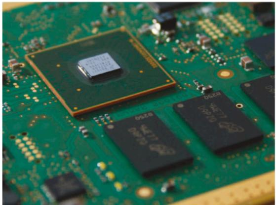
Industrial grade SBC Qseven module built on **Freescale LS1021A** based on dual ARM Cortex-A7 cores.
